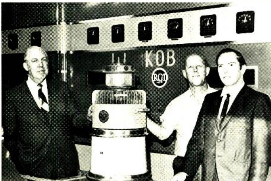
KOB transmitter tube is pulled from service after 15 years and 108,000 hours of operation. Left to right, George S. Johnson, KOB-AM research director, J. Beverly, Transmitter CE, and Fern Bibeau, KOB Operations CE.
